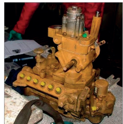
A fuel pump worn out by cavitation
