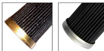
Varnish coated in-line filter of IGV servo valve
