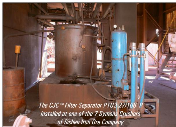
*The CJC™ Filter Separator PTU3 27/108 P installed at one of the 7 Symons Crushers of Sishen Iron Ore Company*
