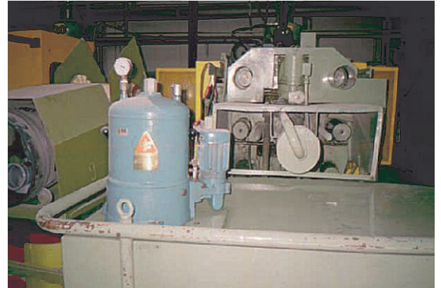
At Wavin Metalplast in Buk, Poland all STORK plastic injection moulding machines are equipped with CJC™ Fine Filters.
